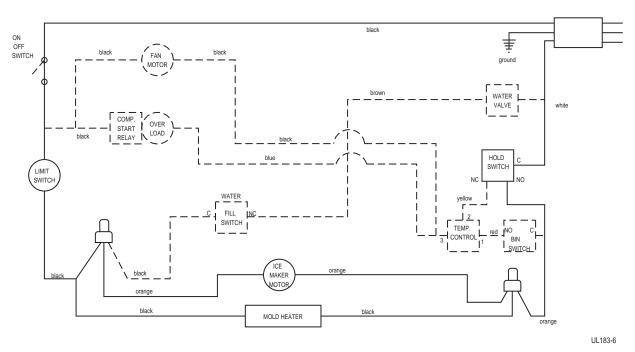
HARVEST-2 CYCLE (Hold Switch In Switched Position)
